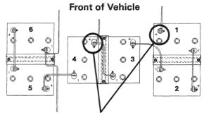
Remove these battery cables before working on vehicle.
